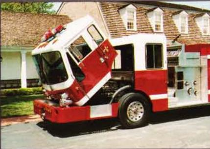
45° cab tilt provides generous access to engine and components. Dual sealing surfaces and hidden rain tunneling provide positive protection against water and noise without the problems and costs of pneumatic seals.
