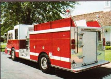
The massive rear compartment holds rescue tools or cascade systems with easy working access. Rear access to stokes basket, back boards and ground ladders can be built in with low ground proximity.
